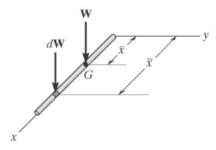
Consider the 1-dimensional rod in the figure, with total weight W acting on the center of gravity  $\bar{x}$ . If we take an infinitesimally small segment with weight dW at an arbitrary location  $\tilde{x}$ , then we can determine the total weight mathematically by:
