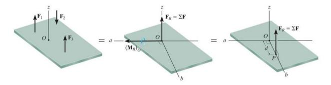
If  $\vec{F}_R$  and  $(\vec{M}_R)_O$  are perpendicular to each other, they can be further simplified by placing  $F_R$  at a distance *d* from the moment, which is found by:
