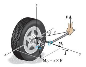
In this example, the force creates a moment about an axis in the xy-plane. But in order to determine the rotation that will actually unscrew the lug, the rotation about the y-axis is required.
