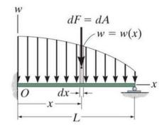
Consider a one-dimensional beam subjected to a distributed load, as shown. If we take an infinitesimally small element of the load, the force acting on that element is:
